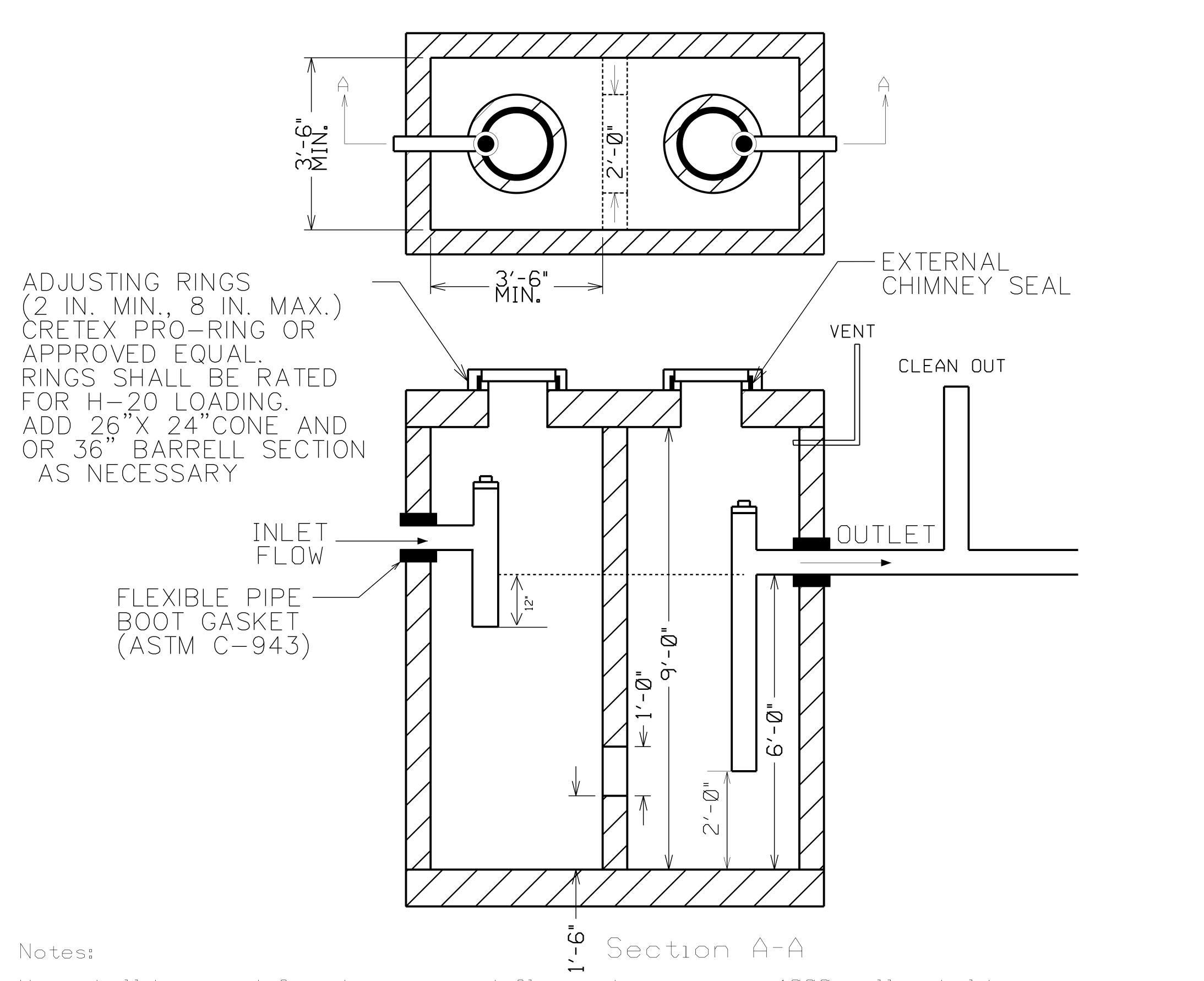
Unit shall be sized for the expected flow with a minimum 1000 gallon holding capacity. Interior minimum length of each compartment shall be 42".
