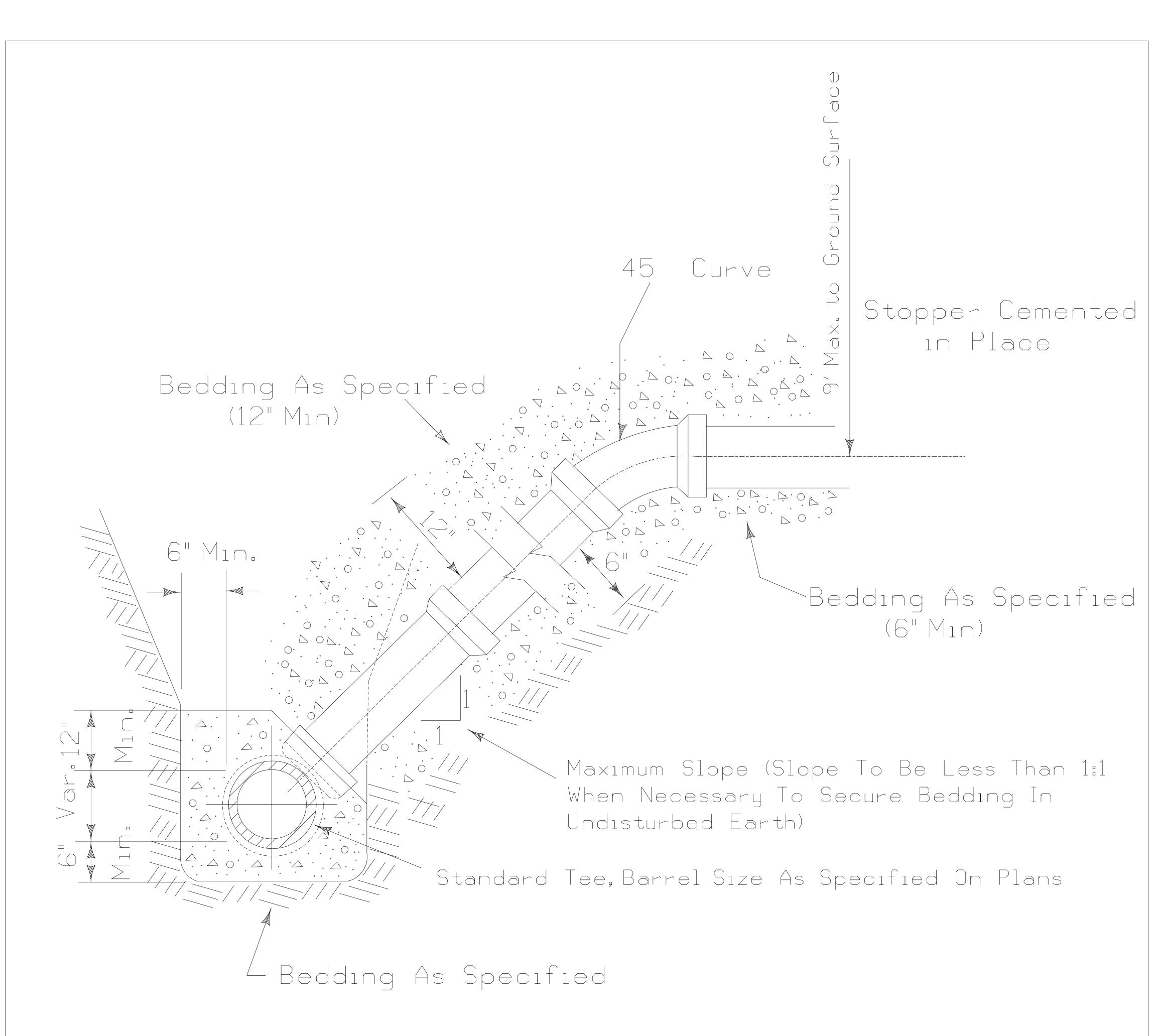
Note : Sanıtary Connection on Existing Mains shall be ROMAC "CB" OR FORD Sewer Saddle ASTM A 536, ASRM D 2000 MBA 710,
