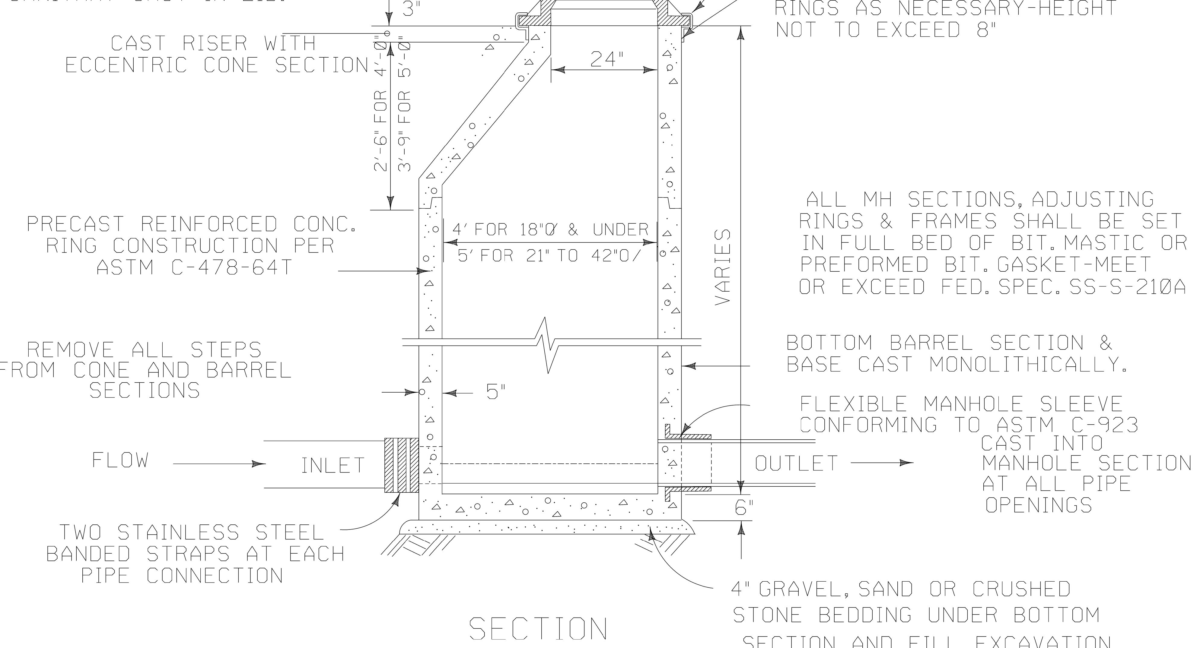
NOTE: EXTERNAL BAND TO BE INSPECTED JUST PRIOR TO ANY PAVING OPERATIONS.
