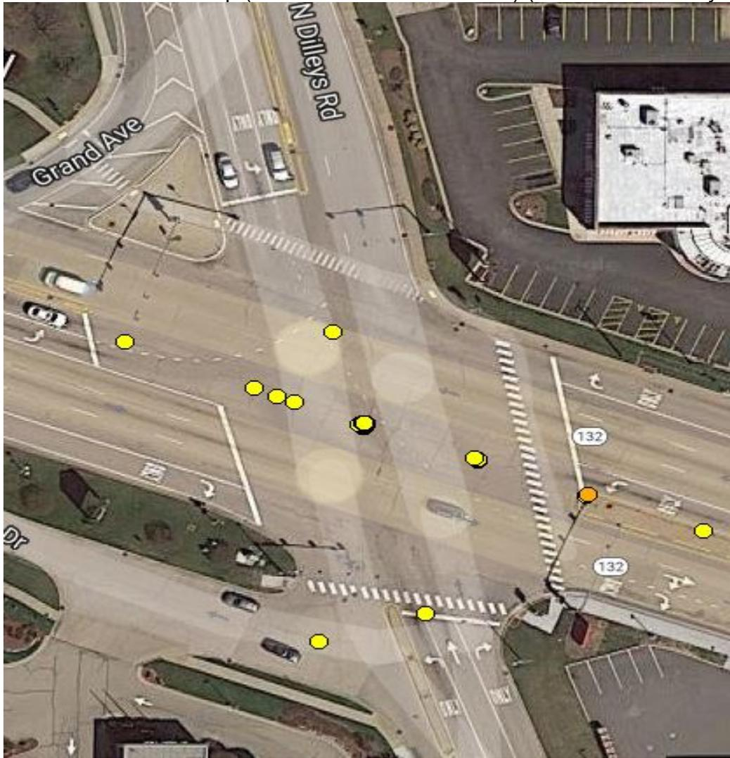
2007 Collision Diagram (Data located on Exhibit #1) (Route 132 & Dilleys)
