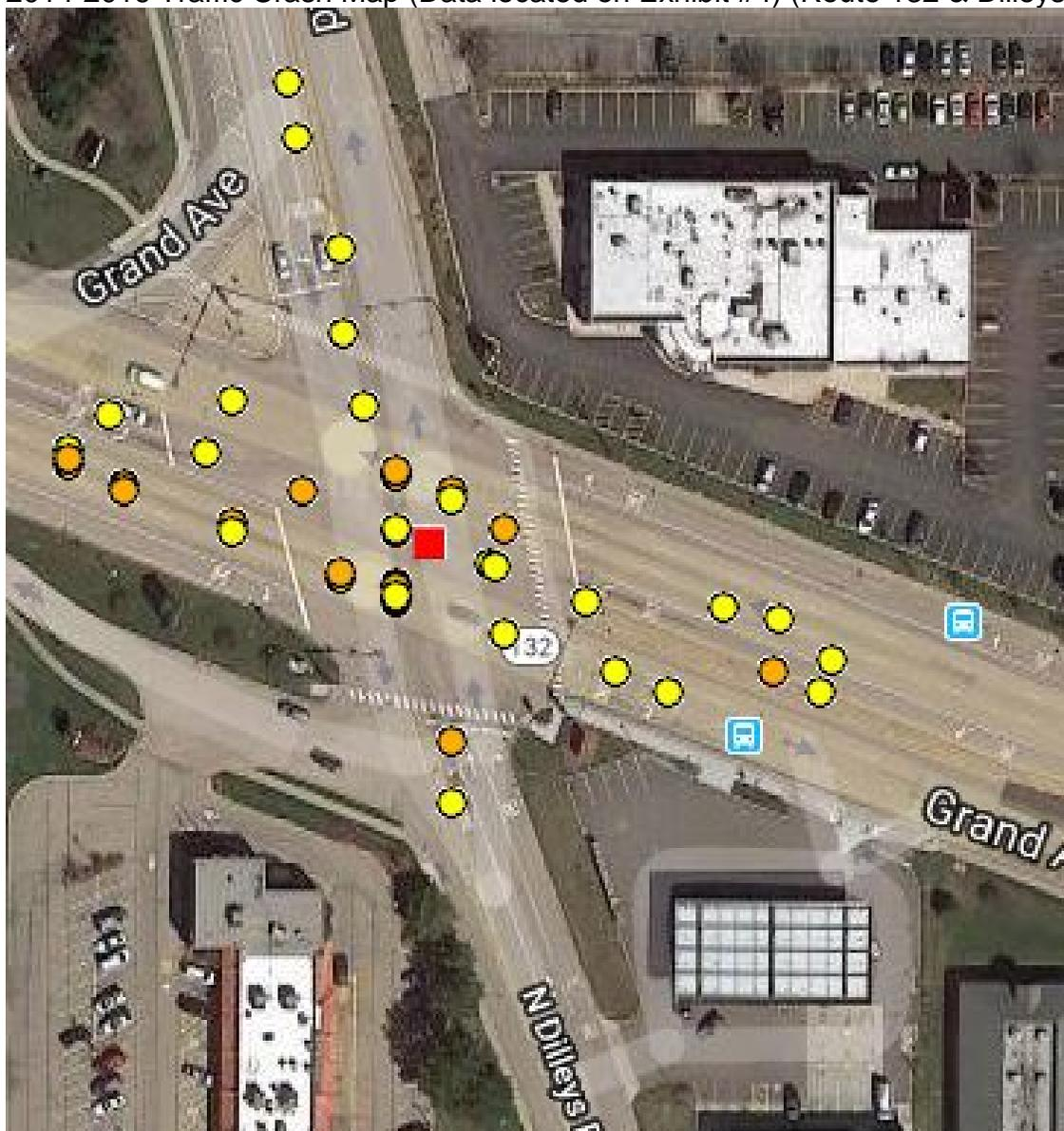
2014-2016 Collision Diagram (Data located on Exhibit #4) (Route 132 & Dilley's)
