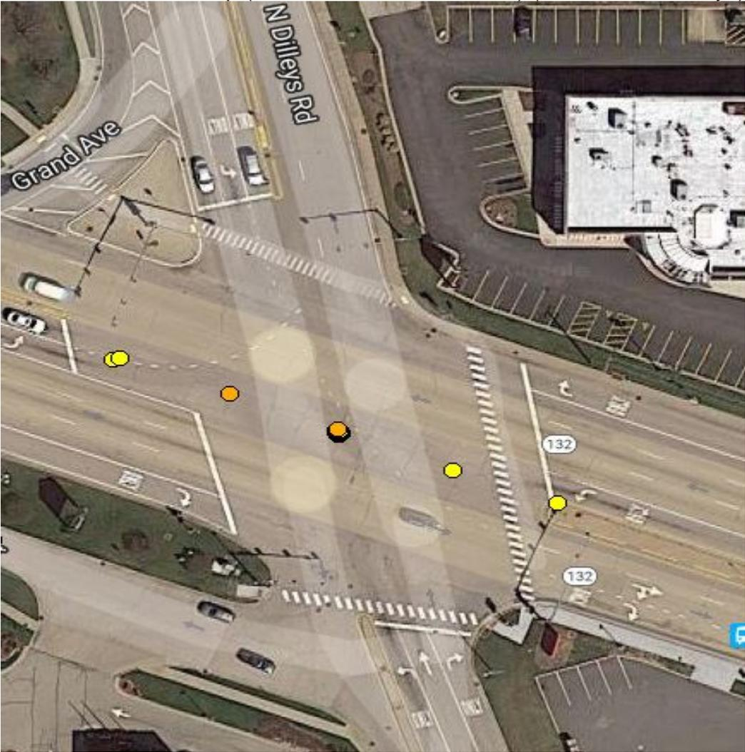
2006 Collision Diagram (Data located on Exhibit #1) (Route 132 & Dilleys)
