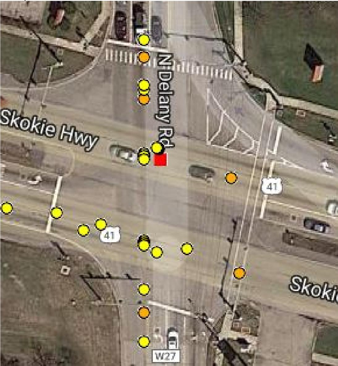
2014-2016 Collision Diagram (Data located on Exhibit #5) (Route 41 & Delany Road)
