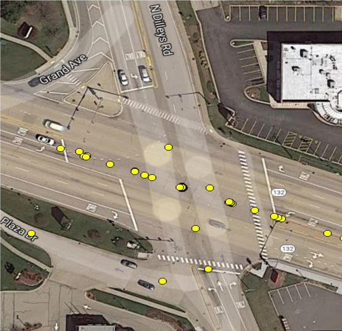
2006-2008 Collision Diagram (Data located on Exhibit #1) (Route 132 & Dilleys)
