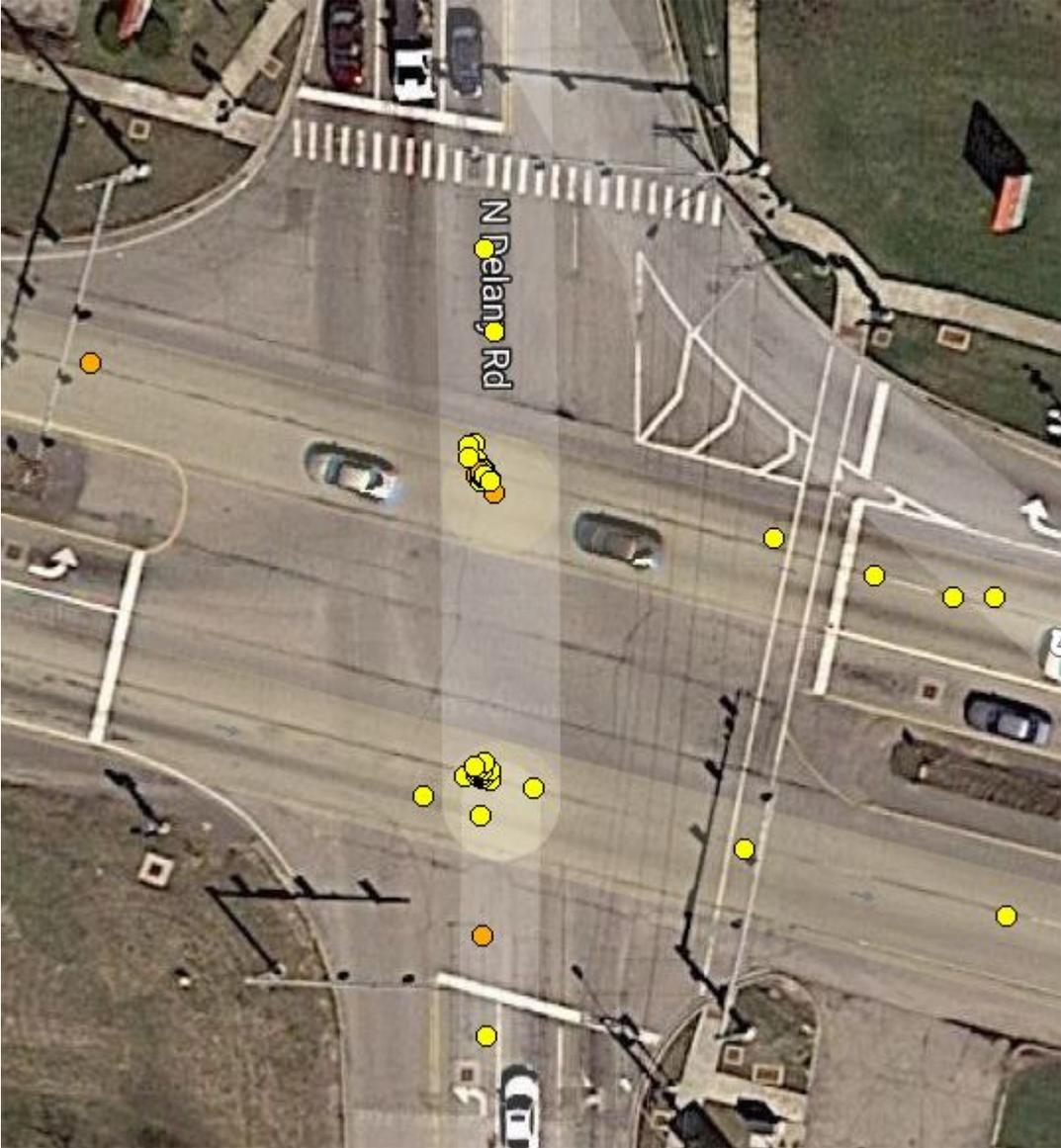
2006-2008 Collision Diagram (Data located on Exhibit #1) (Route 41 & Delany Road)
